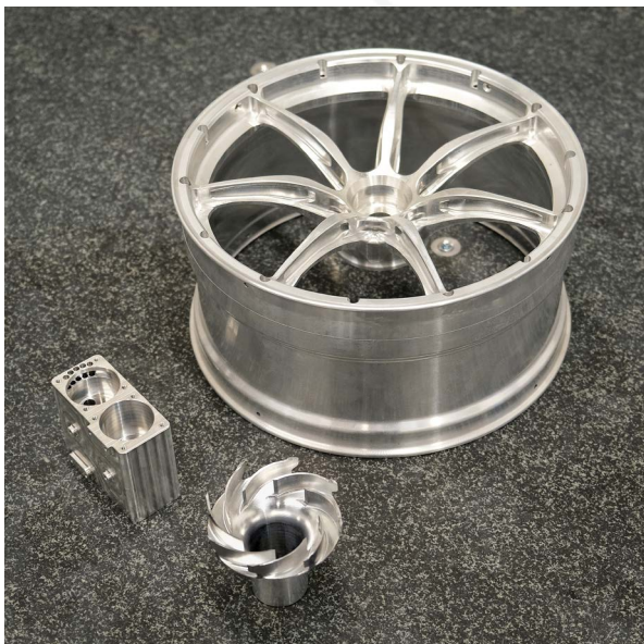
Typical components, all machined from solid aluminium, inspected by Driven Engineering on the LK CMM: clockwise from back, the scaled-down race car wheel, an impeller and an aircraft fuel pump component
